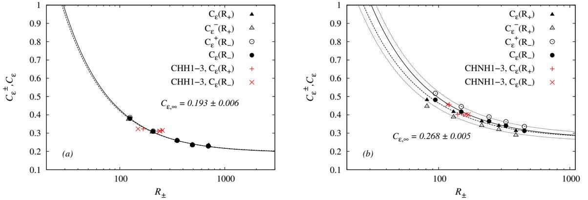
FIG. 2. The solid lines show the model equations for  $C_\epsilon$ ,  $C_\epsilon^+$  and  $C_\epsilon^-$  fitted to data for (a) series CH06H and (b) series CH06NH with initial relative cross helicity  $\rho_c(0) = 0.6$ . The red crosses refer to additional runs with  $0.2 \leq \rho_c(0) \leq 0.8$ .
