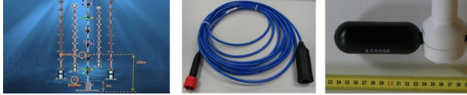
Fig. 9. View of the ANTARES neutrino telescope (left) and pictures of the emitter FFR SX30 (middle) and of the receiver HTI-08 (right) transducers.
