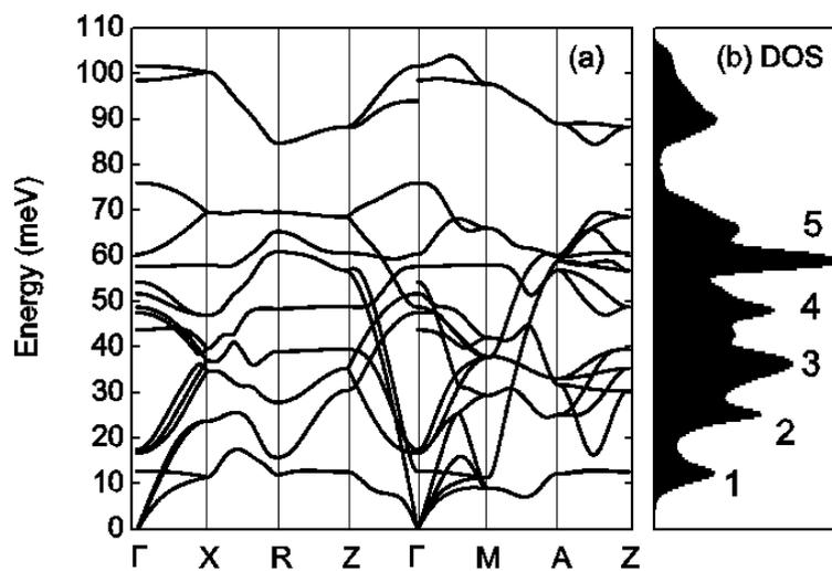
FIG. 7. (a) Calculated phonon dispersion of rutile TiO<sub>2</sub> along the high symmetry directions. (b) The corresponding phonon DOS. The DOS peaks are labeled by the same numbers as those in Fig.1 of the paper
