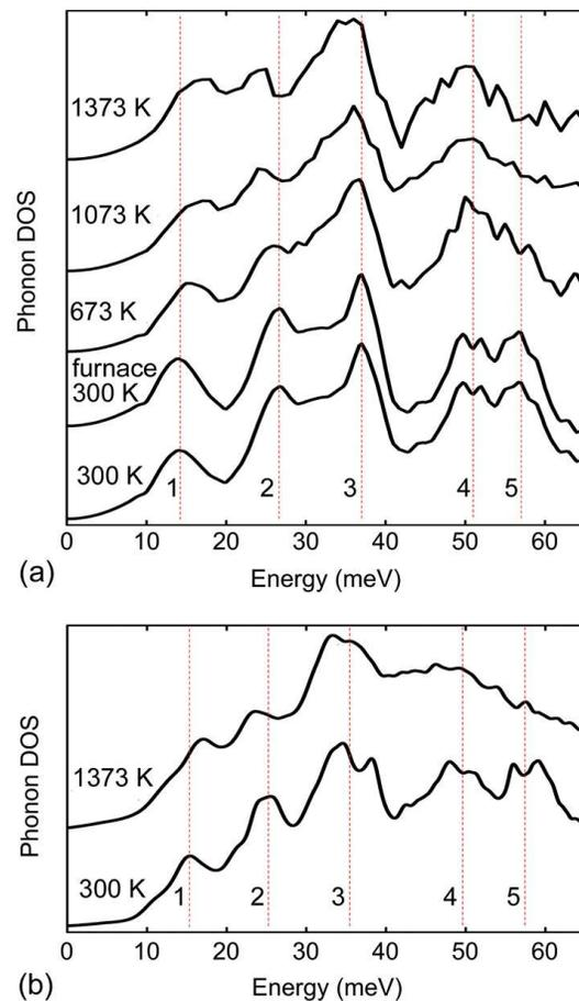
FIG. 2. (a) Neutron weighted phonon DOS of rutile  $\text{TiO}_2$  from measurements at temperatures from 300 to 1373 K with an incident energy of 75 meV. Five vertical lines are aligned to peak centers at 300 K. (b) Phonon DOS of rutile  $\text{TiO}_2$  at temperatures of 300 and 1373 K calculated with first principles MD simulations and the FTVAC method.
