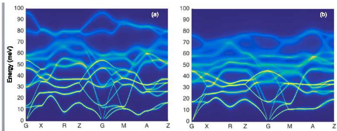
FIG. 8. TDEP phonon spectra along high symmetry points at (a) 300 K and (b) 1373 K
