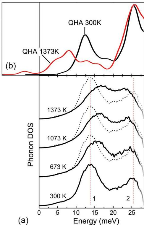
FIG. 3. (a) Neutron weighted phonon DOS of rutile  $\text{TiO}_2$  from measurements at temperatures from 300 to 1373 K with an incident energy of 30 meV (so data above 26 meV are less reliable). The dashed spectrum corresponds to the experimental result at 300 K, shifted vertically for comparison at each temperature. (b) Simulated total phonon DOS from the QHA at 300 K (black) and 1373 K (red).
