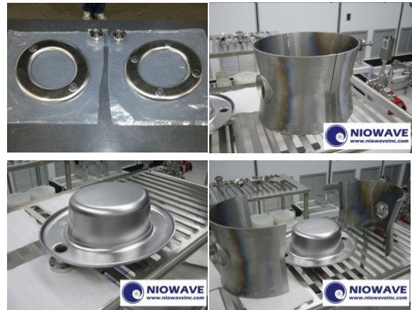
Figure 7. Cavity body fabrication, top-left: top and bottom caps; top-right: outer tube; bottom-left: capacitive plate welded to the inner tube and cap; bottom-right: parts before welding.
