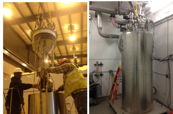
Figure 11. Left: rigging the cavity into the dewar, right: the dewar with cavity inside the SVTF.
