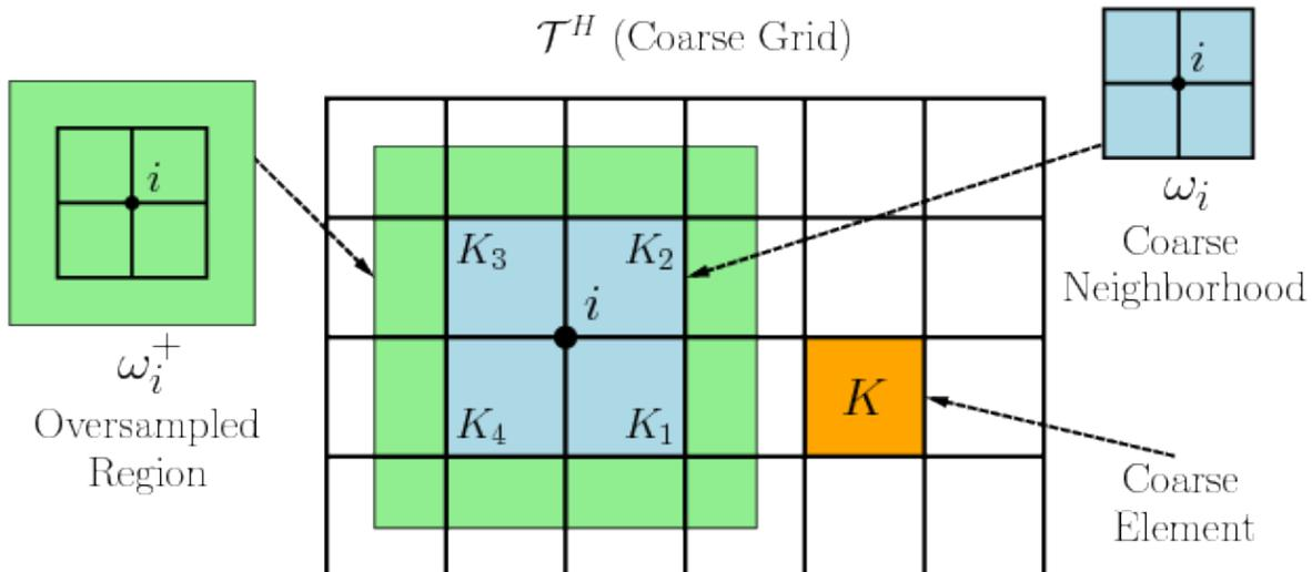
Figure 14: Illustration of a coarse neighborhood and oversampled domain. Here,  $K$  is a coarse-grid block,  $\omega_i$  is a coarse neighborhood of  $x_i$ , and  $\omega_i^+$  is an oversampled region
