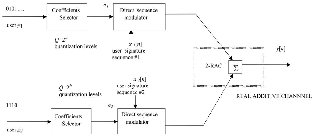
**Fig. 1.** Direct eigensequences transmission system for two users over the 2-RAC. User signature sequences are DFTISs of length  $N$ , belonging to the subspaces of real eigenvalues  $\pm 1$ . The coefficient selection is made by a  $b$  bits D/A converter.
