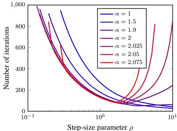
Figure 6. We run Algorithm 2 for eighty-five values of  $\alpha$  evenly spaced between 0.1 and 2.2 and fifty values of  $\rho$  geometrically spaced between 0.1 and 10. We plot the number of iterations required for  $z_k$  to reach within  $10^{-6}$  of a precomputed reference solution. We show only a subset of the values of  $\alpha$  to keep the plot manageable. We omit points corresponding to parameter values for which Algorithm 2 exceeded 1000 iterations.
