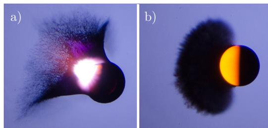
FIG. 1. (Color online) Laser pulses ( $\lambda = 532$  nm) impacting from the left on magenta-dyed water drops of radius  $R_0 = 0.9$  mm. Images are taken  $30 \mu\text{s}$  after impact with a color camera and diffusive backlight illumination. (a) White plasma glow [27] and violent ablation from the drop induced by a focused laser beam. (b) Fluorescence of the dye and ablation at the drop surface due to local boiling induced by a uniform laser irradiation.
