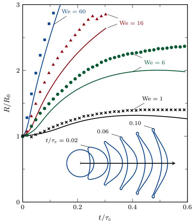
FIG. 6. (Color online) Radial expansion of the drop: experiments (markers) and BI simulations (solid lines). The corresponding image sequences are shown in Fig. 3. The inset shows the drop shape evolution from BI for  $We = 60$  with an exaggerated center-of-mass displacement to separate the successive shapes. The simulations are stopped when the local sheet thickness becomes too thin to resolve the dynamics accurately.
