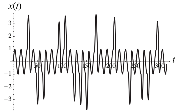
FIG. 25. One realization of the solution to the stochastic equation (7.1) when the noise-free system is in the vicinity of a first-order dynamical phase transition from a phase with a single symmetric solution to a phase with three stable (noise free) steady state solutions, one symmetric about x = 0 and a pair of skewed solutions. The restoring force is provided in Appendix A with \alpha = 0.01, k = 2, F_0 = 0 . Other parameters: drive amplitude, A = 1.89 , frequency, \omega = 0.5 , noise correlator, \Gamma = 0.0001 .
