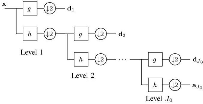
Figure 2: Wavelet analysis filter bank. The signal is iteratively decomposed through a filter bank to obtain its discrete wavelet transform.
