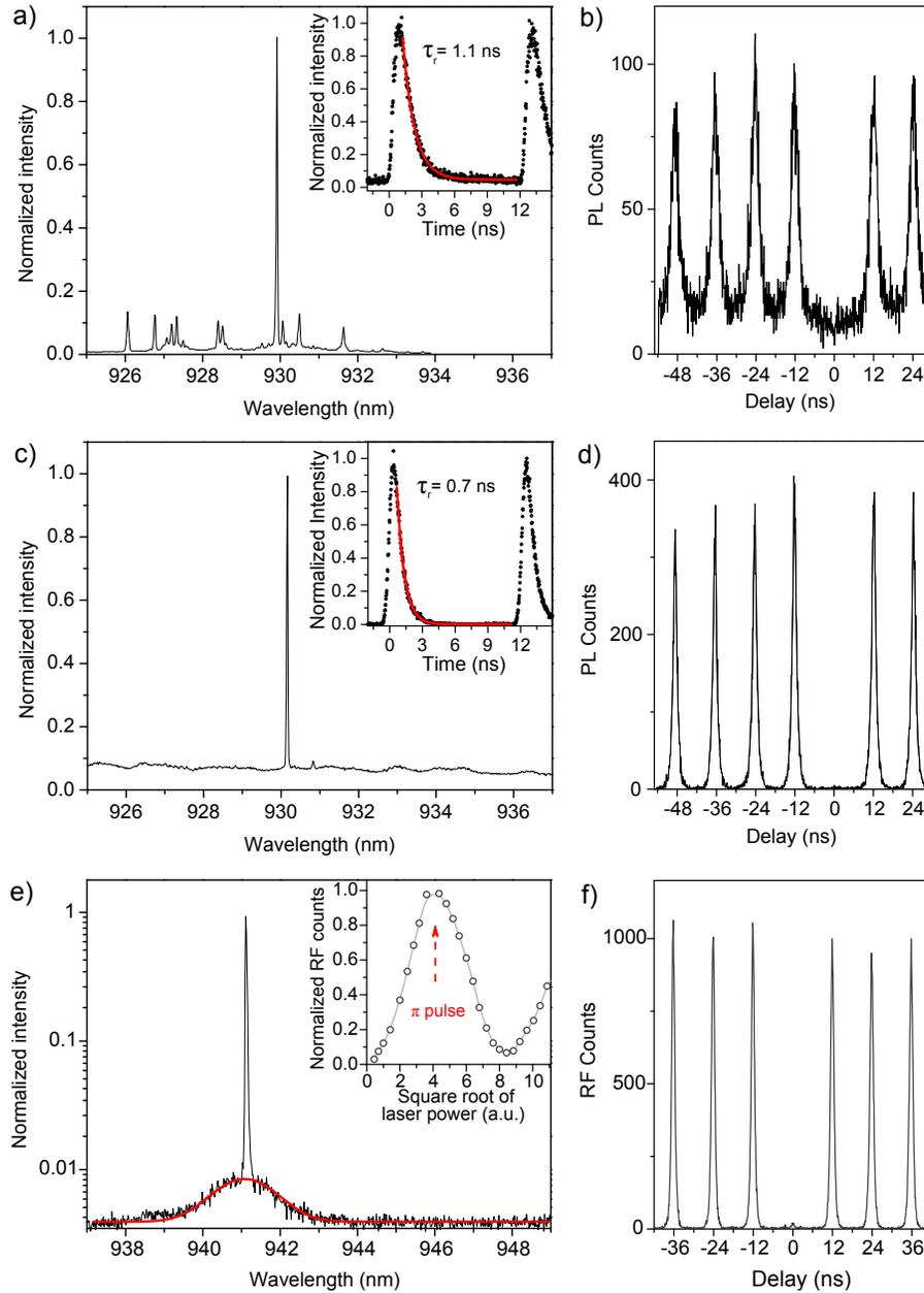
**Fig. 5** a) Photoluminescence (Inset: Time resolved PL) signal of a QD under non-resonant excitation; c) quasi-resonant excitation; e) resonance fluorescence. The inset in e) depicts the power dependency of the emission under pulsed resonance fluorescence, which is characterized by the occurrence of distinct Rabi-oscillations. Corresponding second order correlation histograms: b) non-resonant pumping, d) p-shell excitation; f) resonance fluorescence.).
