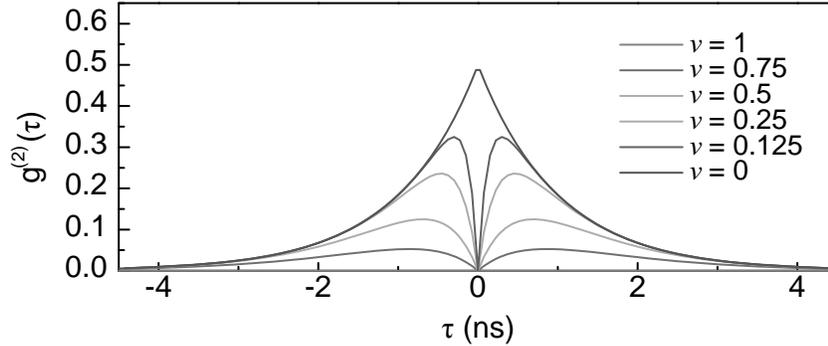
**Fig. 2** Calculated correlation function  $g^{(2)}(\tau)$  of the  $\tau = 0$ -Peak for the interference of indistinguishable photons with a radiative decay time of  $\tau_r = 1$  ns for different visibilities  $v = \tau_c/2\tau_r$ .
