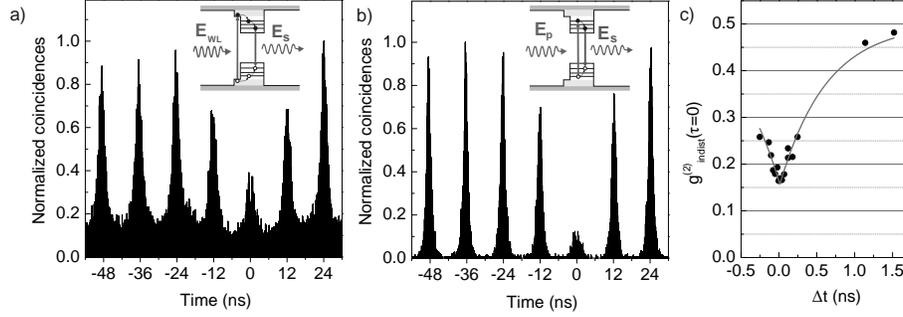
**Fig. 6** a) Two photon interference histogram for a QD. The emitter is non-resonantly excited into the wetting layer. b) TPI under p-shell excitation. c) The Hong-Ou-Mandel dip evolves when the TPI visibility is plotted against the delay time  $\Delta t$ .
