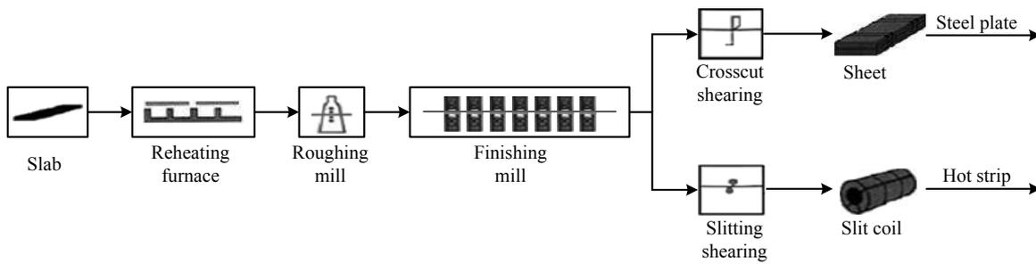
**Fig. 1** A process flow diagram of the hot rolling production procedure
