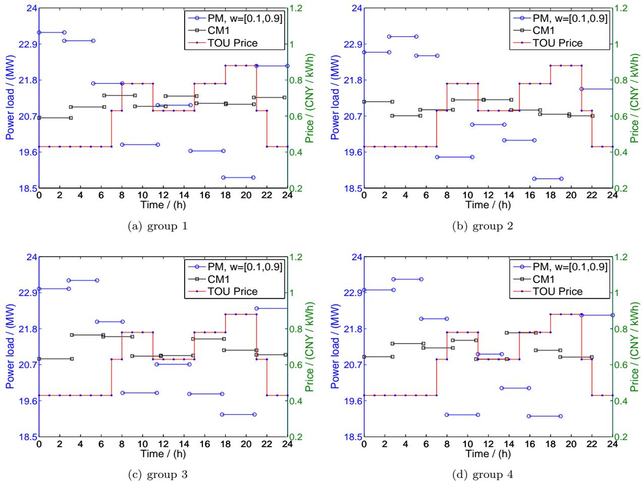
**Fig. 5** Illustration of job scheduling results obtained by PM and CM1
