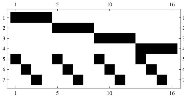
FIG. 2: Pictorial matrix representation of a local area network at Bell Labs (black squares represent ones, white squares represent zeros - see [23, 27]), composed by four subnetworks (fdi, corp, local and switch) communicating via a router. The network topology we consider yields 7 observed aggregate traffic volumes and 16 origin-destination traffic volumes.
