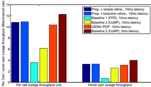
Figure 6: Outage throughput comparisons of different schemes. The number of users in each cell is  $K_0 = 8$  and the number of users per cluster is  $K_c = 4$ . The other simulation setup is the same as the basic simulation setup.
