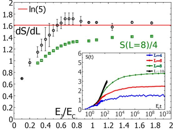
Fig. 6: Entropy per spin in thermodynamic limit extrapolated to  $t = \infty$ . The insert shows  $S(t)$  dependence in the bad metal regime at  $E_J/E_C = 0.3$  that shows slow relaxation of the entropy to its saturation value.
