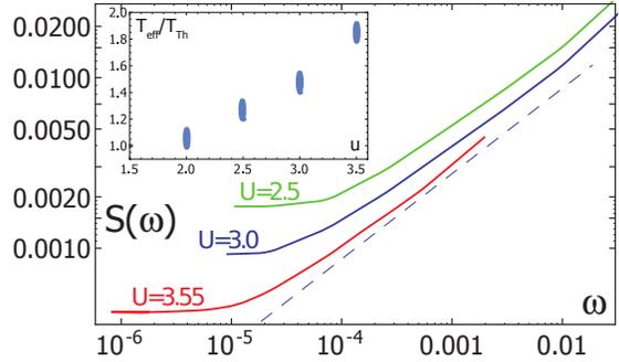
Fig. 5: Spectrum of current noise fluctuations,  $S(\omega)$  for different internal energies,  $U = 2.5, 3.0, 3.55$ . The dashed line shows  $S(\omega) \sim \omega^{1/2}$  dependence. Insert shows the effective temperature determined from FDT relation.
