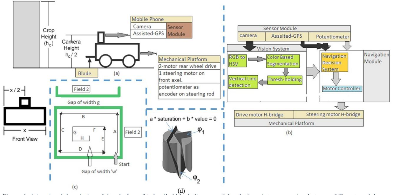
Figure 1: (a) a visual description of the platform (b) detailed block diagram of the platform interconnection between different modules (c) the model case considered for the control and navigation algorithms (d) the HSV cylinder for subspace decomposition
