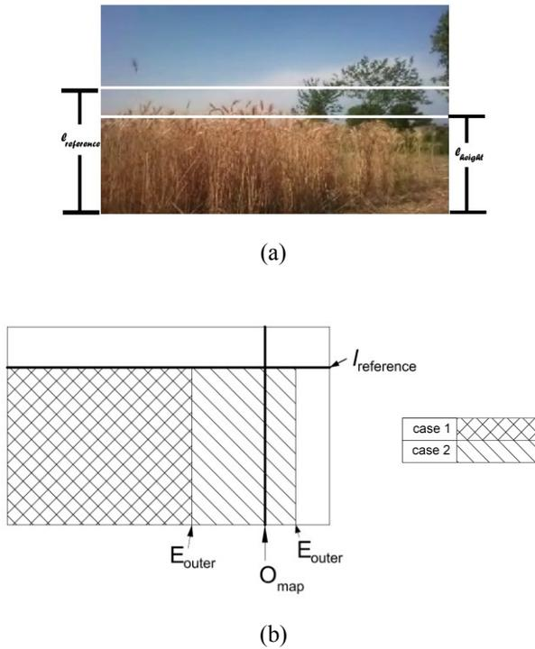
**Fig 2: Demonstration of vehicle navigation using the imaginary reference line and offset: (a) detection of end of field through the difference between the reference line and the top of the crop in the next field; (b) adjustments in vehicle path depending on the outer crop boundary, case 1:  $E_{outer}$  is to the left of  $O_{map}$ , case 2:  $E_{outer}$  is to the right of  $O_{map}$ .**
