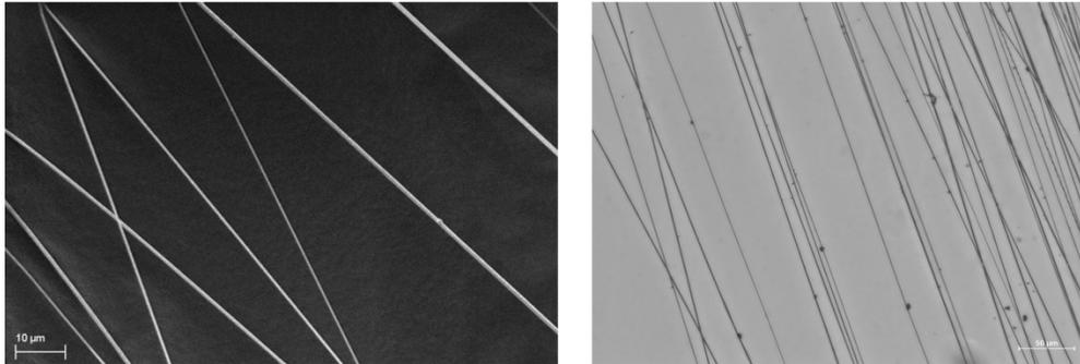
Figure 2 (a-b): Scanning electron microscope image of electrospun fibers with laminin coating (a), and optical microscope image of nanofibers suspended in HA hydrogel (b).
