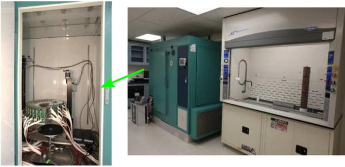
Fig. 1. A dedicated plant PET imager (Left) seats inside a growth chamber (right). A fume hood adjacent to the plant growth chamber and lead lined radioactive gas delivery lines are used for radio-tracer administration.
