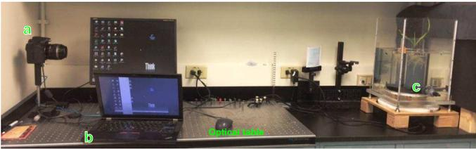
Fig. 2. Optical imaging system: (a) DSLR camera; (b) controlling laptop for synchronizing object rotation and image capturing; (c) water tank and rotation stage for optical imaging.
