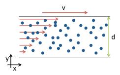
FIG. 1. (Color online) Shear cell with periodic boundary conditions along flow direction. The reflecting walls on the top and bottom are separated by a distance d. The top wall moves at constant speed v in the x direction, while the bottom wall is fixed, causing a linear gradient  $\dot{\gamma} = v/d$  in the solvent flow velocity along the y direction.
