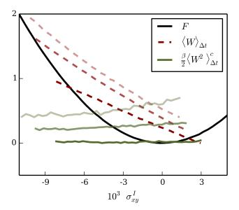
FIG. 3. (Color online) Using the method illustrated in Figure 2, we compute  $\langle W \rangle_{\Delta t}(\sigma_{xy}^I)$  and  $(\beta/2)\langle W^2 \rangle_{\Delta t}^c(\sigma_{xy}^I)$  for a range of values of  $\sigma_{xy}^I$ , and plot this data for Pe values 4, 10, and 19, increasing from bottom to top. Also plotted is the free energy F extracted from the Pe = 0 simulation run.
