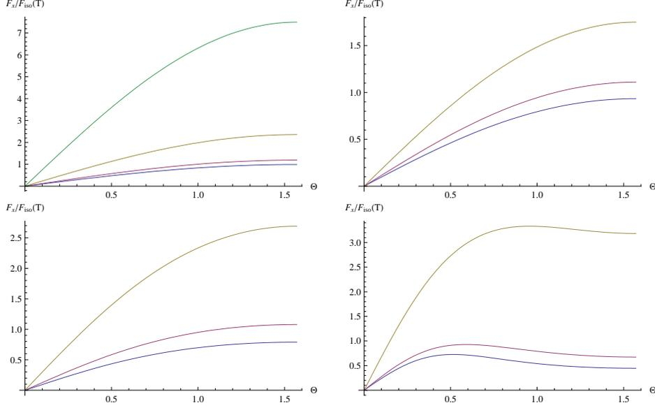
Figure 2: Drag force in  $x$ -direction  $F_x$  as a function  $\Theta$  at  $v = 0.5$ . The four graphs denote  $a/T = 1.38$ ,  $a/T = 4.41$ ,  $a/T = 12.2$ ,  $a/T = 86$  respectively, where the colour lines denote  $Q = 5$  (Green),  $Q = 2$  (Brown),  $Q = 1$  (Red),  $Q = 0$  (Blue).
