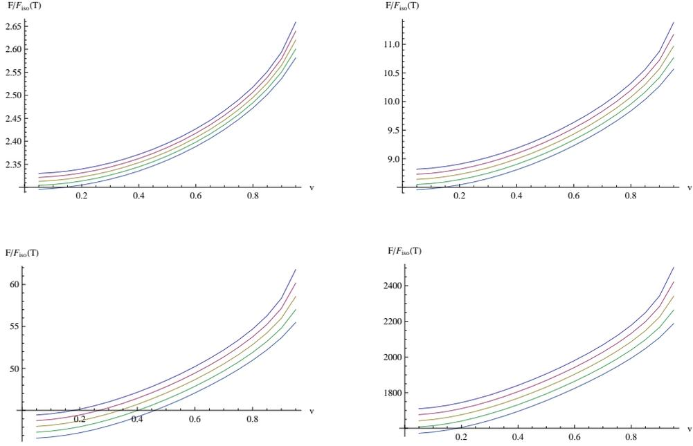
Figure 10: The drag force  $F$  as a function of velocity for a quark moving through the plasma with  $Q = 5$ . The four graphs correspond to  $a/T = 1.38, a/T = 4.42, a/T = 12.2, a/T = 86$  respectively, in which five lines denotes (from the top to down )  $\Theta = 0, \Theta = \pi/6, \Theta = \pi/4, \Theta = \pi/3, \Theta = \pi/2$
