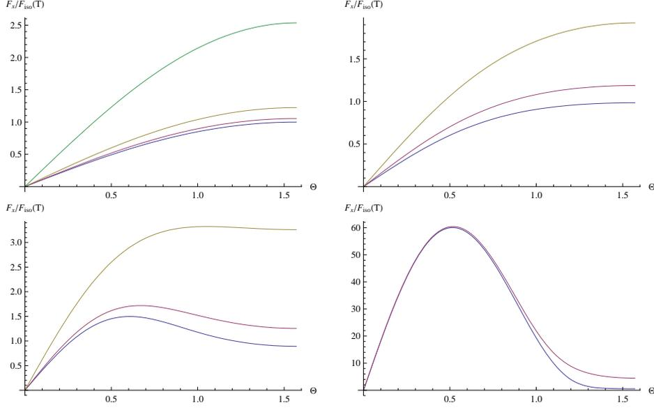
Figure 3: (color online) Drag force in  $x$ -direction  $F_x$  as a function  $\Theta$  at  $v = 0.9$ . The four graphs denote  $a/T = 1.38$ ,  $a/T = 4.41$ ,  $a/T = 12.2$ ,  $a/T = 86$  respectively. where the colour lines denote  $Q = 5$  (Green),  $Q = 2$ (Brown),  $Q = 1$ (Red),  $Q = 0$ (Blue).
