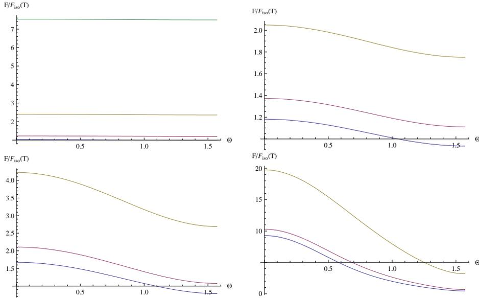
Figure 6: Drag force  $F$  as a function  $\Theta$  at  $v = 0.5$ . The four graphs denote  $a/T = 1.38$ ,  $a/T = 4.41$ ,  $a/T = 12.2$ ,  $a/T = 86$  respectively, where the colour lines denote  $Q = 5$  (Green),  $Q = 2$ (Brown),  $Q = 1$ (Red),  $Q = 0$ (Blue).
