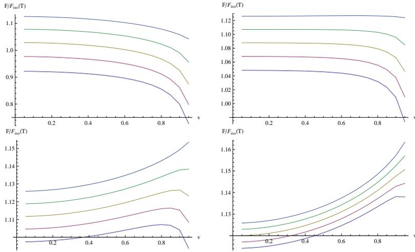
Figure 15: Drag force  $F$  as a function velocity  $v$  for  $T = 0.3$ . The four graphs correspond to  $Q = 0.5, 2, 5, 10$  respectively, in which the five lines denote  $\Theta = 0, \pi/6, \pi/4, \pi/3, \pi/2$  from the bottom to top.
