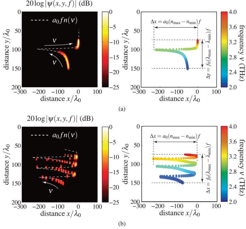
Fig. 7: Normalized wave intensity  $|I(x, y, f)|$  computed with (11) showing 2-D frequency scanning in the output plane for uniformly spaced frequencies within the specified bandwidth in the presence of a dispersive wedge exhibiting a) single resonance, as in Fig. 4(a), and b) multiple resonances, as in Fig. 4(b). Left graphs show the superimposed beam spots of different frequencies while right graphs show the corresponding 3-dB contour plots.
