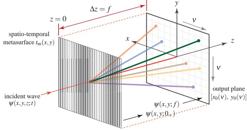
Fig. 2: Spatio-temporal metasurface decomposing the temporal spectrum of a broadband wave,  $\psi(x, y, z; t)$ , in two spatial dimensions, where each frequency  $\nu$  is mapped onto a specific point  $[x_0(\nu), y_0(\nu)]$  in the focal plane at  $z = f$ .
