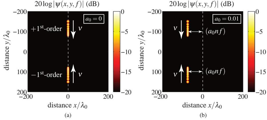
Fig. 6: Normalized wave intensity  $|I(x, y, f)|$  computed with (11) showing 1-D frequency scanning in the output plane for uniformly spaced frequencies within the specified bandwidth a) in the absence of wedge, and b) in the presence of a non-dispersive wedge of refractive index  $n = 3$ . Only one of the two diffraction orders are shown. Each bright spot represents a distinct frequency  $\nu$ .
