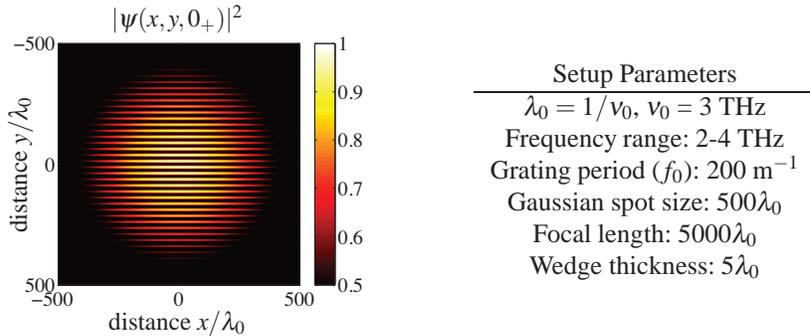
Fig. 5: Normalized wave intensity  $|I(x, y, 0_+)|$  corresponding to Gaussian beam illumination of the wedged diffraction grating (left), and parameters used in the numerical examples (right). The modulation index of the grating is assumed to be  $m = 1$ .
