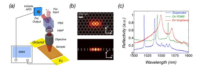
FIG. 2. (a) A schematic of the cross-polarized confocal microscope measurement setup. (b) A Finite-difference time-domain (FDTD) simulation of the cavity energy intensity. (c) Reflection spectra of the PPC cavity suspended over SOI substrate (blue), on PDMS substrate (green) and on the dual-layer graphene capacitor (red).
