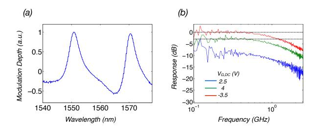
FIG. 4. (a) Modulation depth as function of input laser wavelengths measured at 3 kHz (b) High frequency response of the graphene modulator at different DC gate voltages. Dotted lines indicate the response of 0 dB and -3 dB.
