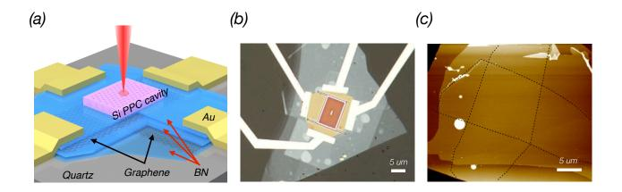
FIG. 1. (a) Schematic of the cavity-graphene electro-optic modulator. The dual-layer graphene capacitor on quartz substrate is optically coupled to the PPC cavity. (b) Optical image of fabricated cavity-graphene electro-optic modulator. (c) AFM image of the BN-graphene-BN-graphene-BN five-layer stack. Two graphene layers (black dashed line) are pristine and sandwitched in the BN layers.
