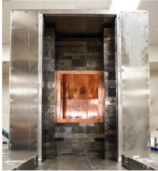
Figure 2: Low background copper and lead shielding of the MAJORANA DEMONSTRATOR inside the anti-radon enclosure.
