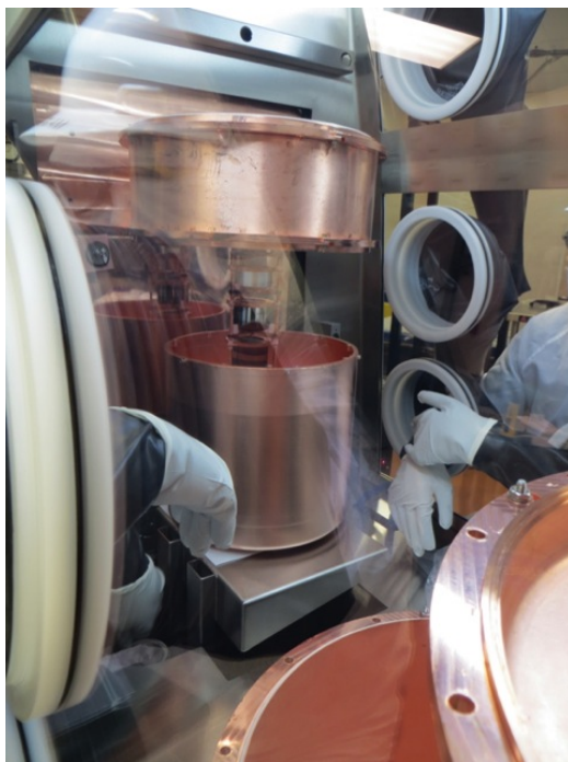
Figure 3: Prototype Cryostat during the strings installation.
