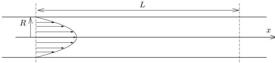
FIG. 9. Poiseuille flow: the time of flight is calculated with Poincaré sections being separated by a length L .
