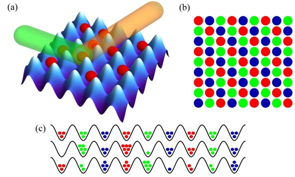
FIG. 1. (a) Setup: light is scattered from atoms in an optical lattice. Generated spatial structure of 3 matter-field modes in 2D (b) and 1D (c) lattice. Sites of the same colour are indistinguishable to light scattering and thus belong to the same mode. The superposition of three indistinguishable atom distributions in (c) is protected by light scattering.
