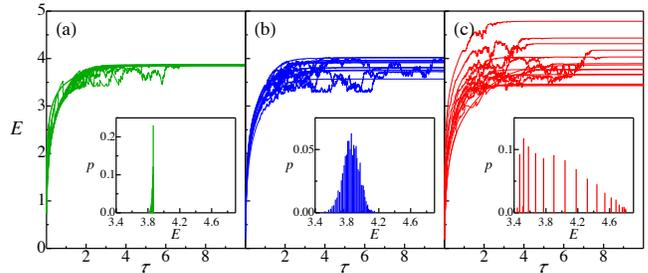
FIG. 2. Quantum trajectories for the growth of entanglement between two modes where the detected variables are (a) atom number difference in diffraction minimum; (b) total atom number in diffraction maximum; (c) absolute value of atom number difference in minimum. Insets show the final entanglement distribution functions.  $\langle N \rangle = 50$ ,  $\tau = 2|C|^2 \kappa t$ .
