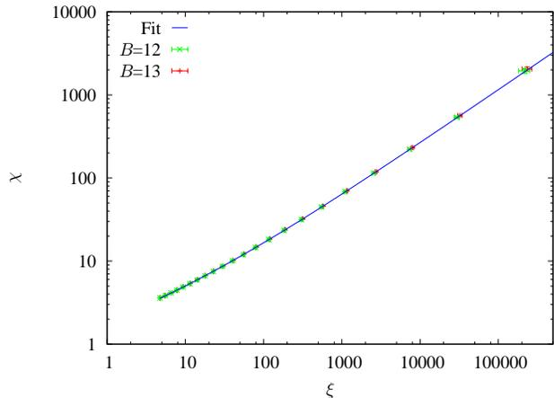
FIG. 4: (color online) Extrapolated thermodynamical susceptibility  $\chi$  versus  $\xi_2$  for  $\rho = 5/3$ . The two data sets correspond to extrapolations obtained by using up to  $B = 13$  data (red points) and up to  $B = 12$  data (green points).
