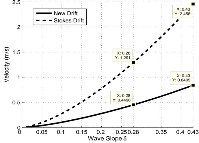
Figure 4: Comparison between the newly derived wave drift and Stokes drift respect to a surface wave with amplitude  $A = 2\text{m}$  along with the variation of wave slope  $\delta$ .
