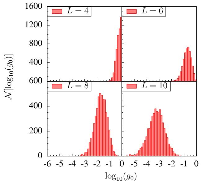
FIG. 1: (Color online) Histogram of the number of samples with fraction in the ground state  $g_0$  at  $\beta = 5$  for various sizes  $L$ , estimated from the reference runs described in Table I.  $\mathcal{N}[\log_{10}(g_0)]$  is the number of samples in the logarithmic bin centered at  $\log_{10}(g_0)$ . There are a total of 50 bins. Note that as  $L$  increases, the histograms shift rapidly to smaller values.
