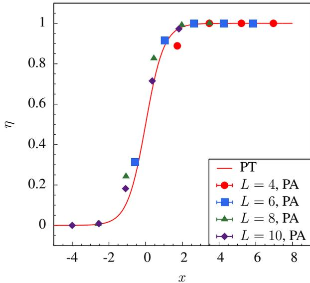
FIG. 7: (Color online) Fraction of samples for which the ground state is found ( $\eta$ ) as a function of the scaled computational work  $x$  [Eq. (13)] for both population annealing and parallel tempering. The curve is taken from the empirical fit [Eq. (12)] of Ref. [23].
