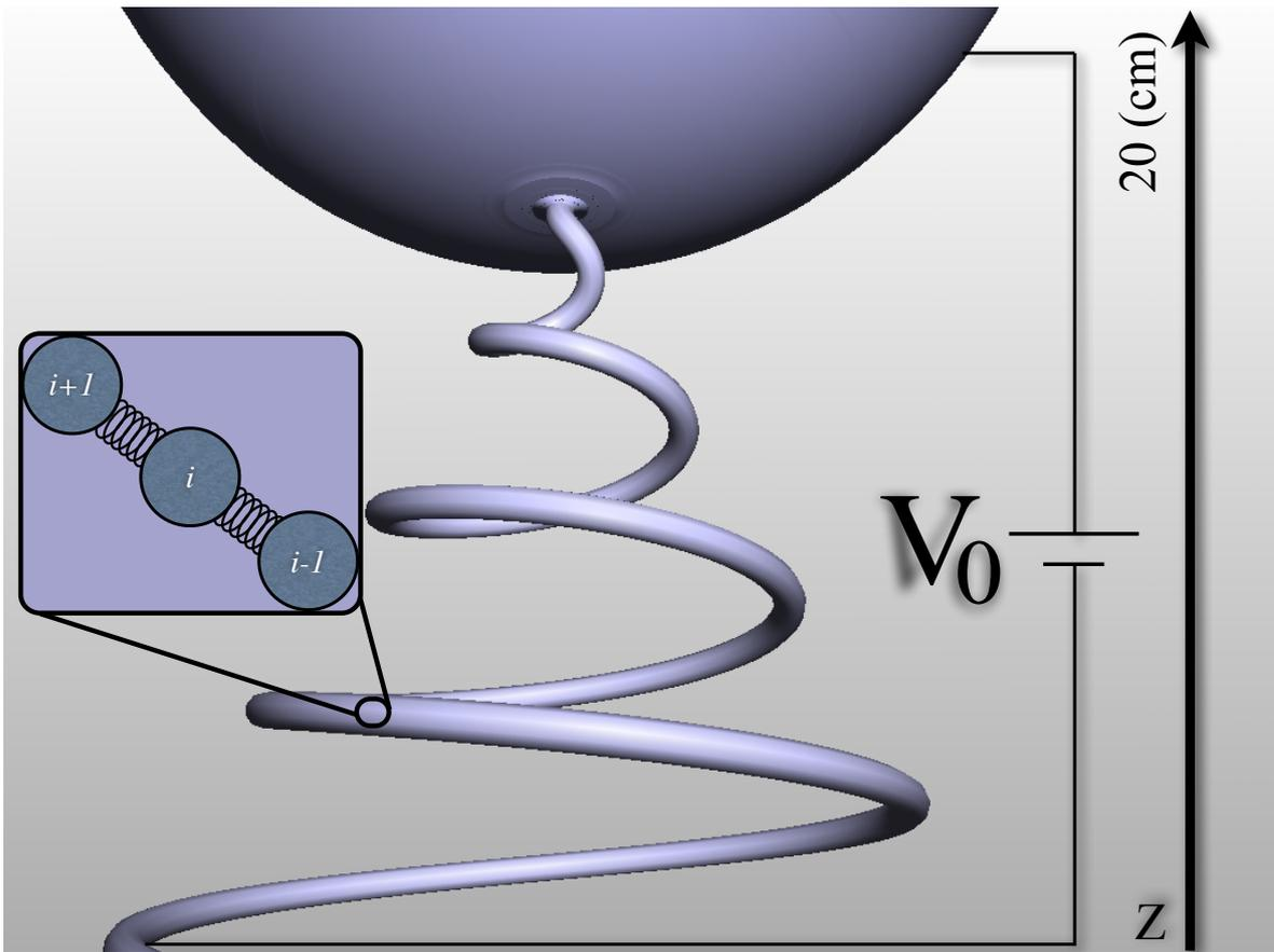
Figure 1. Schematic representation of the model for the polymer jet. The jet is generated from the pendant drop on the top of the figure upon application of the external field  $V_0/h$ . The jet is then represented at a microscopic level as a bead-spring chain. Each bead is charged while the connecting springs are calculated by solving the associated polymer stress equations at each molecular dynamics time step.
