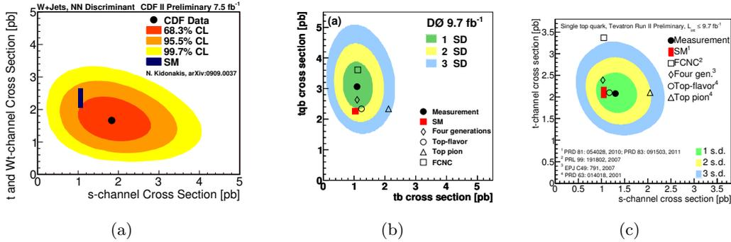
**Figure 4.** Posterior density as a function of t-channel and s-channel single top cross section for CDF l+jets analysis (a), for D0 analysis (b) and the Tevatron single top combination (c).
