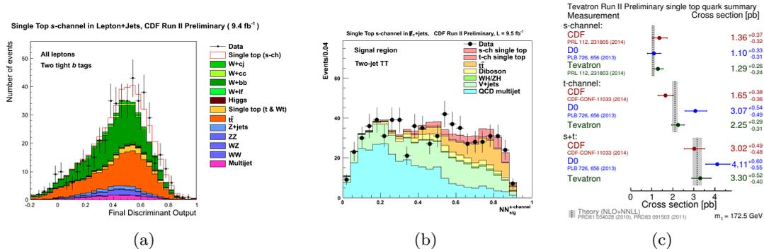
**Figure 5.** s-channel final discriminant in the CDF lepton+jets analysis (a) and  $E_T$ +jets analysis (b). Summary of the Tevatron single top quarks cross section measurements (c).
