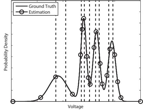
Fig. 5. Channel estimation result at 3000 P/E using Levenberg-Marquardt algorithm and 10-bin equal-probability histogram. (ground truth parameter vector is [0.0099,0.3500,0.0500,0.0617,-0.5882], estimation error vector is  $10^{-4} \times [0.0101 \ 0.0214 \ -0.1774 \ 0.0405 \ -0.0044]$ )
