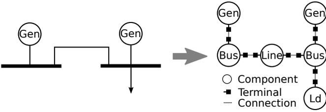
Fig. 1: Conversion to component orientated representation.
