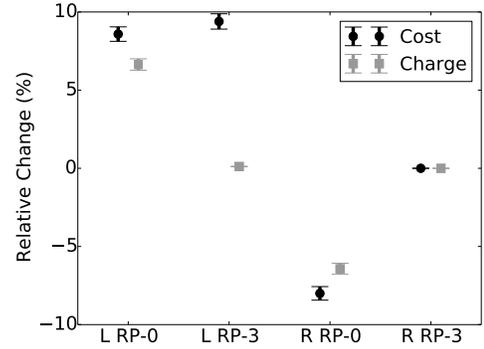
Fig. 4: Performance of cost functions with lowering (L) and raising (R) solar output.
