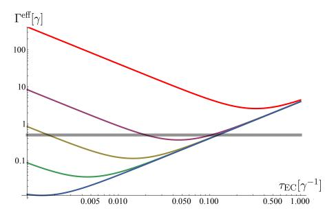
FIG. 6: Log-log plot of the effective decoherence rate  $\Gamma^{\text{eff}}$  versus the error correction time  $\tau_{\text{EC}}$  for different values of the gate error probability  $p_{\text{gate}}$ . The grey line denotes the bare unencoded case, with decay rate  $\gamma/2$ . In decreasing value, these errors are  $p_{\text{gate}} = 5 \times 10^{-2}, 10^{-3}, 10^{-4}, 10^{-5}$  and  $10^{-6}$ .
