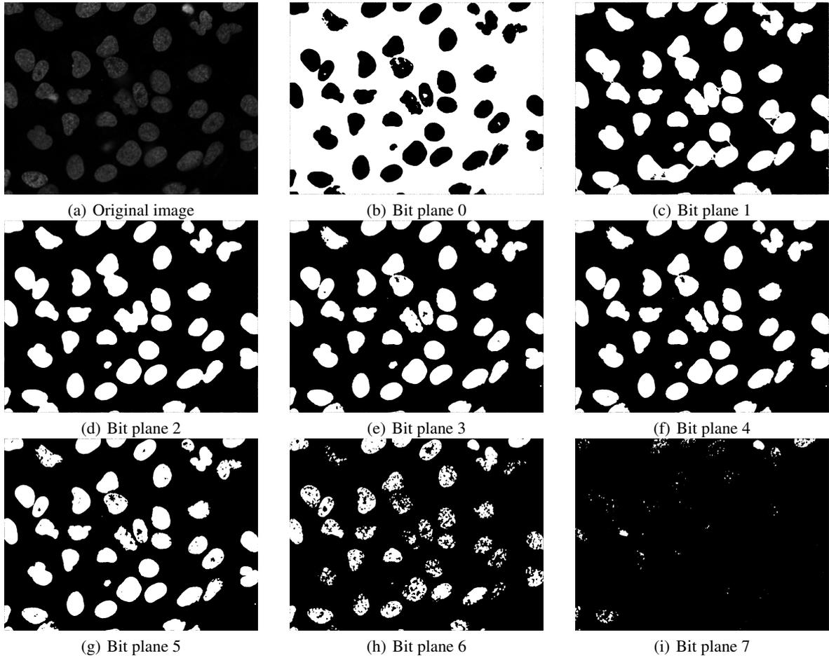
Figure 2: (a): Original image. (b)-(i) bit planes of 2(a).
