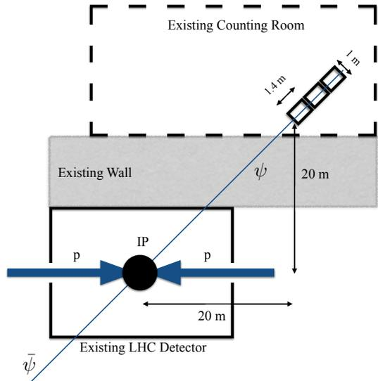
FIG. 3: A schematic showing the experimental setup proposed in this work. Three  $1 \text{ m} \times 1 \text{ m} \times 1.4 \text{ m}$  scintillators, each composed of 200  $10 \text{ cm} \times 5 \text{ cm} \times 140 \text{ cm}$  bars could be deployed in either the ATLAS or CMS counting room. The mCP signal would consist of one or more photo-electrons deposited by the mCP, as it travels through each of the three detector layers, within a narrow timing window from each other.
