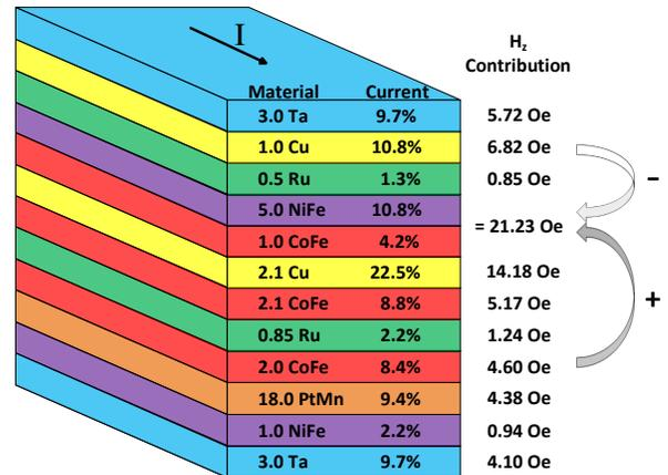
FIG. 2: Current distribution in GMR stack and magnetic field contribution from each layer. Note that the Oersted field contribution from the Cu spacer layer is dominant.
