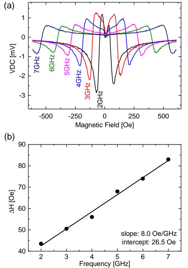
FIG. 6: (a) DC voltage from the spin diode effect as a function of magnetic field for various frequencies at  $\theta = 90^\circ$ , (b) full width at half maximum ( $\Delta H$ ) as a function of frequency.
