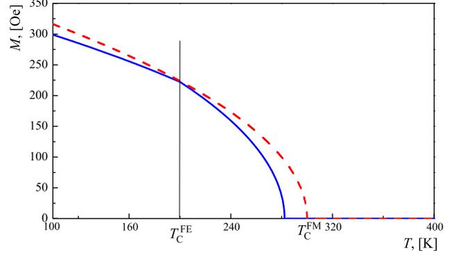
FIG. 8. (Color online) Magnetization  $M$  vs temperature  $T$  for strong spatial dispersion and zero external magnetic and electric fields. Solid (blue) line describes the case of finite interaction of the FE layer with the GFM film while the dashed (red) line corresponds to the non-interacting case.
