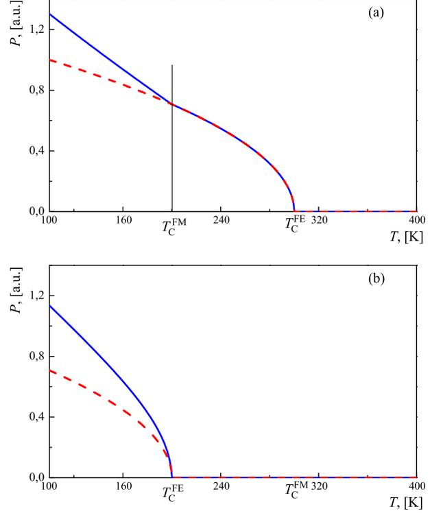
FIG. 7. (Color online) Average polarization  $P$  of the FE layer along the  $z$  direction vs temperature  $T$  at zero external magnetic and electric fields. Solid (blue) line describes the case of finite interaction of FE layer with GFM film. Dashed (red) line corresponds to the non-interacting case. (a) Limit of  $T_C^{\text{FE}} > T_C^{\text{FM}}$  (b) Limit of  $T_C^{\text{FE}} < T_C^{\text{FM}}$ .
