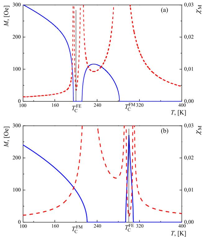
FIG. 4. (Color online) Magnetization  $M$  (solid blue line) and magnetic susceptibility  $\chi_{\text{M}}$  (dashed red line) vs temperature at zero magnetic and electric fields and strong coupling between charge fluctuations and magnetization. (a) Limit of  $T_{\text{C}}^{\text{FE}} < T_{\text{C}}^{\text{FM}}$ , (b) Limit of  $T_{\text{C}}^{\text{FE}} > T_{\text{C}}^{\text{FM}}$ . Two additional phase transitions occur in the vicinity of the FE phase transition.
