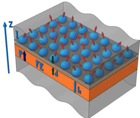
FIG. 1. (Color online) Composite multiferroic - material consisting of granular ferromagnetic film placed at distance  $d$  above the FE layer (FE) of thickness  $h$ . Ferromagnetic film consists of ferromagnetic metallic particles (blue spheres) with finite magnetic moments (red arrows) embedded into an insulating matrix (I). FE layer has a polarization  $P$  along the  $z$ -axis.
