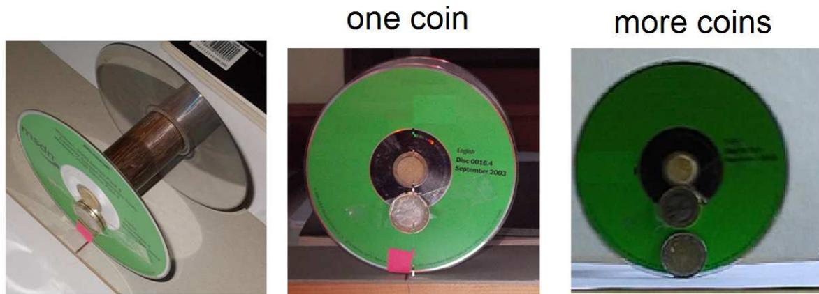
FIG. 1 The rolling spool (made with two CDs and a wooden cylinder) with extra masses (coins) breaking the symmetry of the system.
