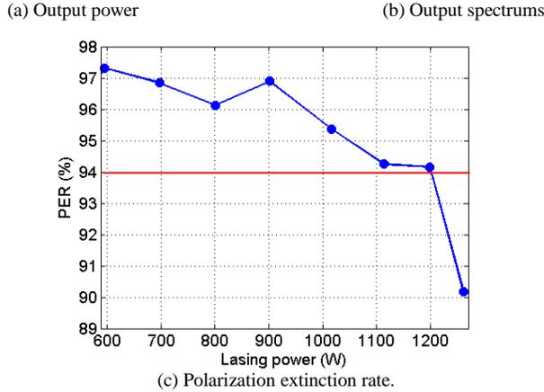
Fig. 2. Output characteristics of the main amplifier.
