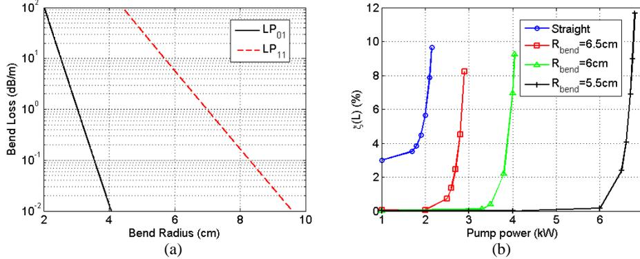
Fig. 6 The effect of coiling on MI threshold power.
