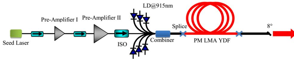
Fig. 1. The architecture of the all-fiber PM amplifier
