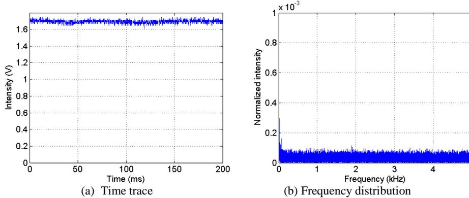
Fig. 7 Fluctuation characteristics of the output beam after tight coiling.
