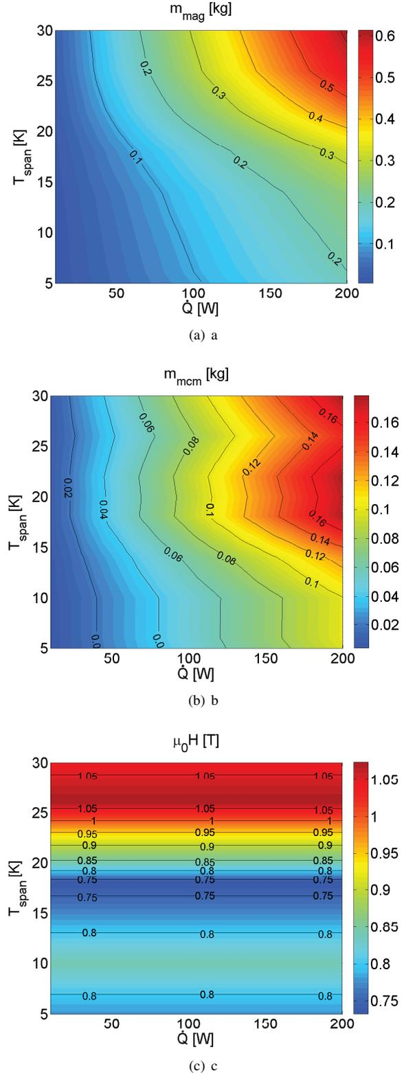
**Figure 5.** (a) The amount of magnet material, (b) the corresponding amount of magnetocaloric material and (c) the corresponding magnetic field for the magnetic refrigeration system with the lowest combined cost of the magnet and magnetocaloric material for a packed bed AMR with Gd and a Halbach cylinder permanent magnet assembly.
