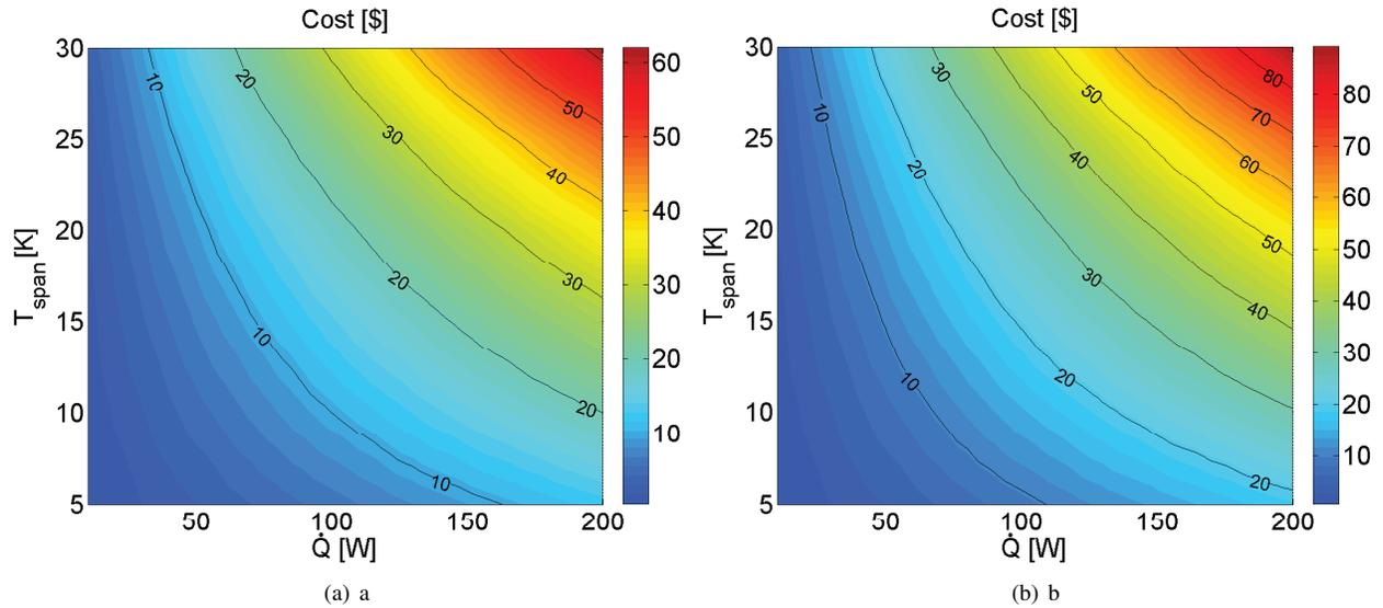
**Figure 6.** The minimum combined cost in \$ of a parallel plate magnetic refrigeration system with a magnetocaloric material with constant  $\Delta T_{ad}$  as a function of temperature span and cooling power for (a) a  $M_{25}$  permanent magnet assembly and (b) a Halbach cylinder of infinite length.
