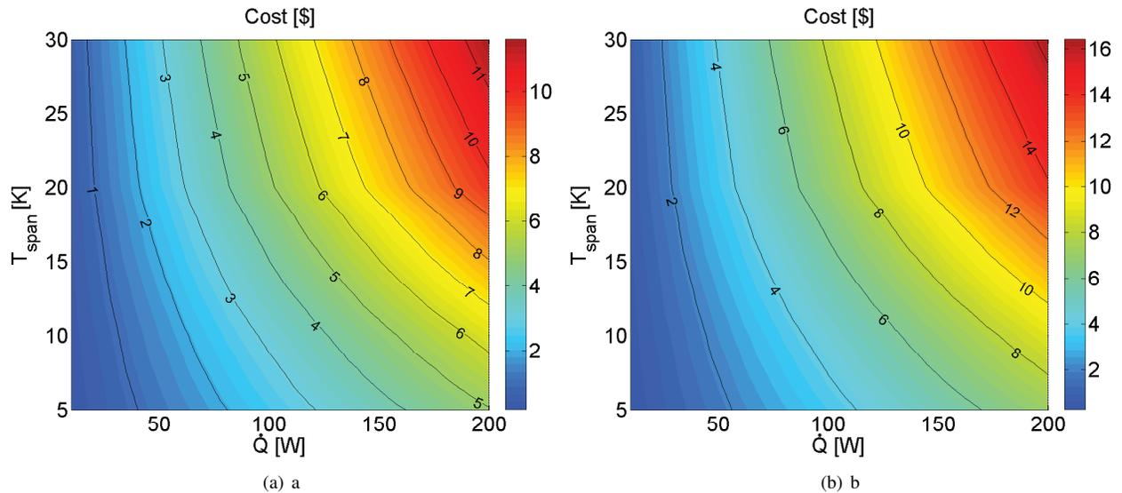
**Figure 7.** The minimum combined cost in \$ of a packed sphere bed magnetic refrigeration system with a constant  $\Delta T_{ad}$  magnetocaloric material as a function of temperature span and cooling power for (a) a  $M_{25}$  permanent magnet assembly and (b) a Halbach cylinder of infinite length.
