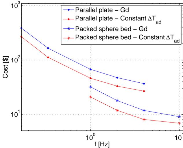
**Figure 9.** The minimum combined cost as a function of frequency for a magnetic refrigeration device using a Halbach magnet and with a temperature span of 20 K and a cooling power of 100 W. The lines are only meant to serve as guides to the eye.
