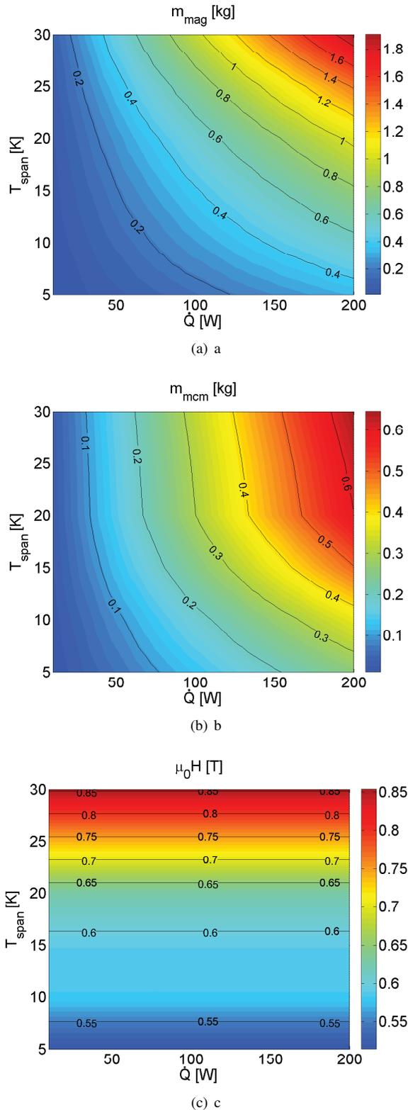
**Figure 8.** (a) The amount of magnet material, (b) the corresponding amount of magnetocaloric material and (c) the corresponding magnetic field for the magnetic refrigeration system with the lowest combined cost of the magnet and magnetocaloric material for a parallel plate constant  $\Delta T_{\text{ad}}$  AMR with a Halbach cylinder permanent magnet assembly.
