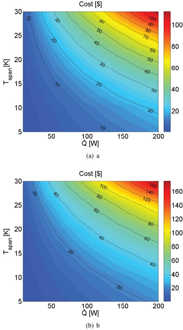
**Figure 2.** The minimum cost in \$ of a parallel plate magnetic refrigeration system of Gd as a function of temperature span and cooling power for (a) a  $M_{25}$  permanent magnet assembly and (b) a Halbach cylinder of infinite length.
