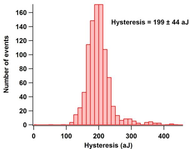
**Figure S4. Hysteresis distribution in hydrogel CRT-MA10\* (n=1000 plots) obtained via AFM force mapping. Hysteresis values were determined from the area bounded between the loading and unloading curves throughout a force map.**
