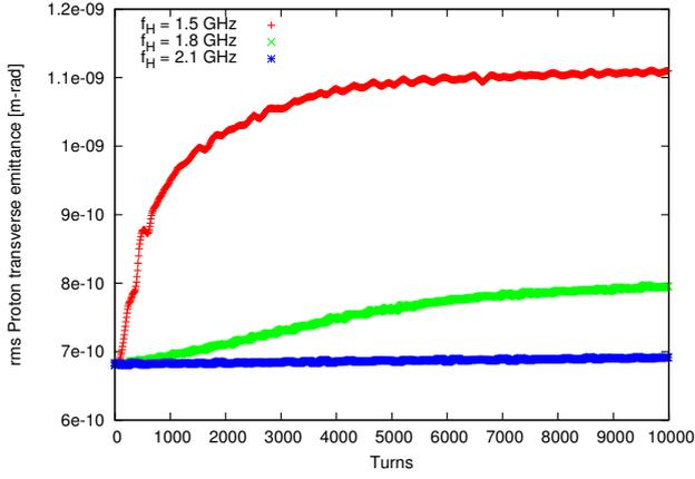
Figure 11: The comparison is shown of kink instability dampings with different high frequency limits  $f_H$  when the disruption parameter  $d_e = 150$ . The gain of the feedback is selected to minimize the emittance growth ion beam.
