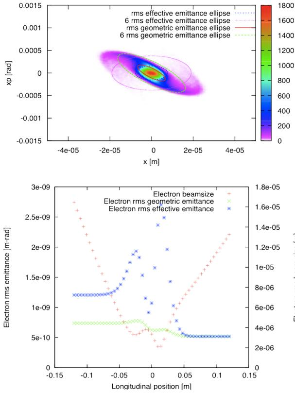
Figure 2: The top figure shows the phase space distribution of the electron beam after collision, and bottom figure shows the evolution of the electron beam size and emittance, for  $d_e = 27$ . In the top figure, the r.m.s. and 6 r.m.s. ellipses for both geometric and effective emittance, respectively, are plotted.
