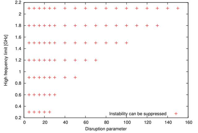
Figure 12: The relation is shown between the required high frequency limit  $f_H$  and the electron disruption parameter  $d_e$ . Each point shows where the instability can be suppressed in the corresponding parameter ( $f_H$  and  $d_e$ ) with proper amplitude. For all calculations, the low frequency limit is set at 50 MHz
