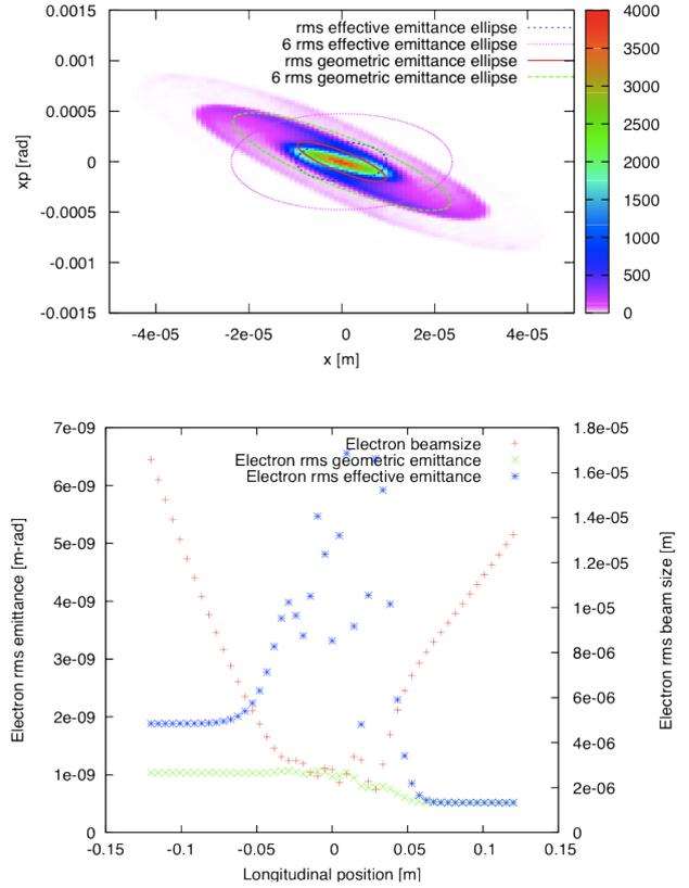
Figure 3: The top figure shows the phase space distribution of the electron beam after collision, and bottom figure shows the evolution of the electron beam size and emittance, for  $d_e = 150$ . In the top figure, the r.m.s. and 6r.m.s. ellipses for both geometric and effective emittance, respectively, are plotted.
