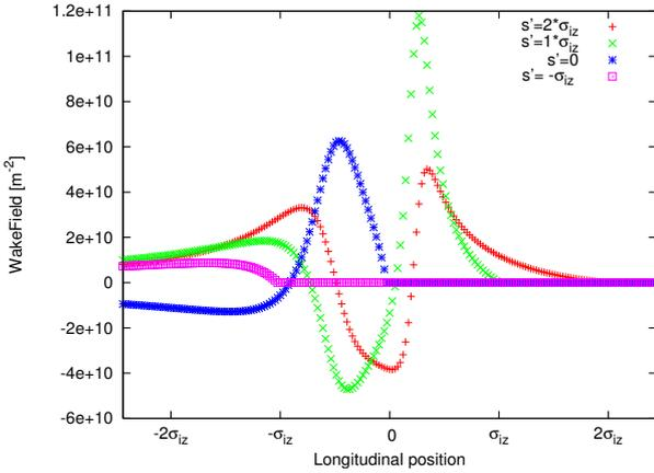
Figure 5: The example of the kink wake field with the beam–beam parameter of the ion beam  $\xi_p = 0.015$  is shown. The electron beam has disruption parameter  $d_e = 27$ . In the figure, the electron beam travels from the positive  $s$  to negative. The symbol  $s'$  denotes the location of the introduced offset.
