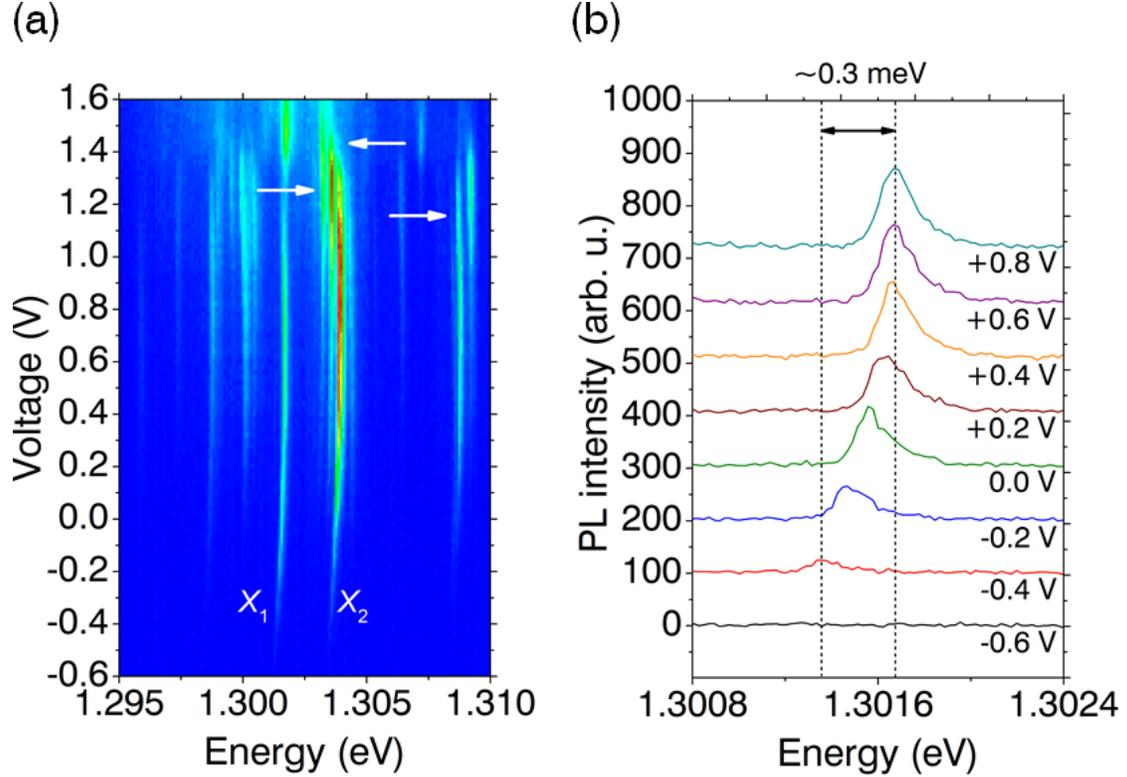
FIG. 2. (Color online) (a) False-color plot of bias voltage dependent single QD emission spectra showing a clear QCSE and charging (marked by arrows). (b) Selected spectra of the  $X_1$  emission for different bias voltages revealing a tuning range of 0.3 meV of the QDs in our samples by the QCSE.
