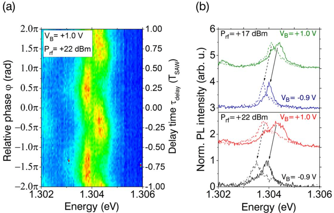
FIG. 4. (Color online) (a) Stroboscopic PL spectra of the  $X_2$  emission line over two full acoustic cycles resolving the *dynamic nature* of the SAW-driven spectral tuning. (b) Independent control of the  $X_2$  emission line by a static electric field and a SAW. The amplitude of the SAW-driven spectral modulation is programmed by  $P_{rf}$  (upper and lower panels) and its center energy can be set by  $V_B$  as shown by the two sets of stroboscopic spectra in each panel.
