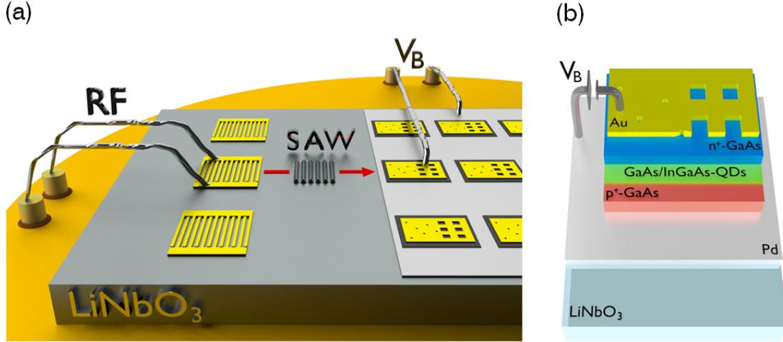
FIG. 1. (Color online) (a) Schematic of our hybrid device consisting of a LiNbO<sub>3</sub> SAW-chip equipped with IDTs and a single QD *pin*-photodiode. (b) Layer sequence of the optically active epitaxially transferred semiconductor film bonded to the LiNbO<sub>3</sub> substrate via a Pd adhesion layer.
