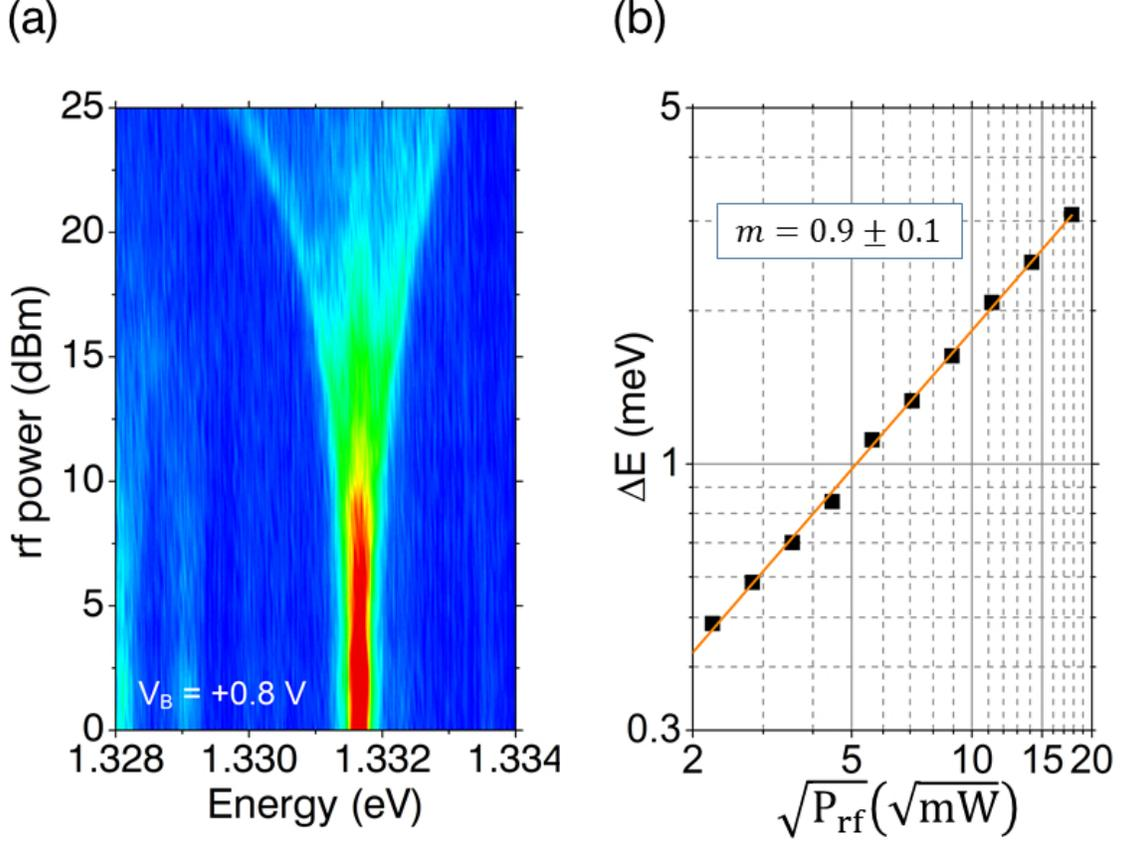
FIG. 3. (Color online) (a) False-color plot of a single QD emission line as a function of  $P_{rf}$  exhibiting a pronounced spectral broadening. (b) Extracted spectral shift  $\Delta E_{DP}$  as a function of  $\sqrt{P_{rf}} \propto A_{SAW}$  revealing a power law  $m = 0.9 \pm 0.1$ , indicative for DP coupling.
