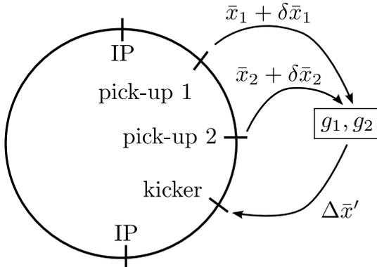
Figure 1: The scheme of the damper model.
