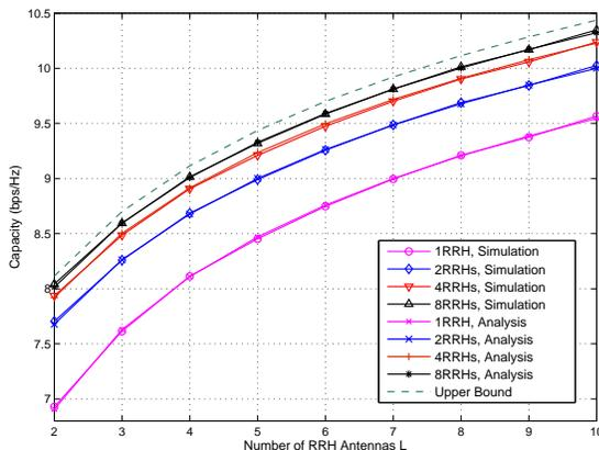
Fig. 2. Ergodic capacity versus antenna number  $L$
