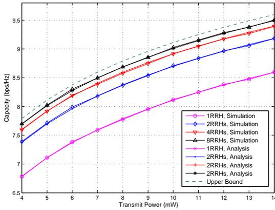
Fig. 1. Ergodic capacity versus transmit power  $P_U$
