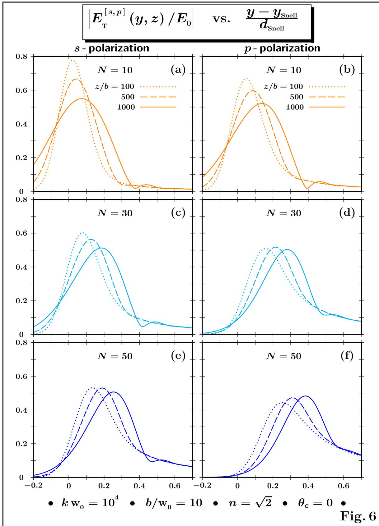
Figure 6: **Focal effect.** For  $k w_0 = 10^4$ , the multiple peaks phenomenon is no longer so evident. Nevertheless, a new interesting phenomenon appears. Due to the second order optical phase contribution, in the outgoing beam can be now observed a focalization effect. This effect is for example clear as in (f).
