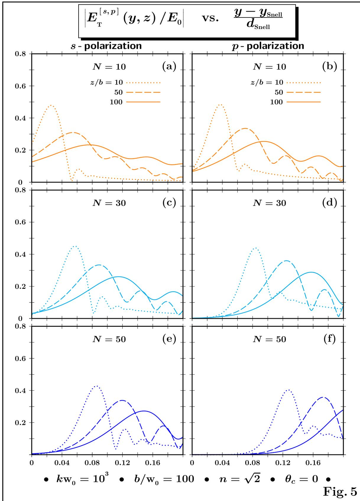
Figure 5: **Multiple peaks phenomenon.** For  $kw_0 = 10^3$ , the outgoing optical beam presents the fascinating phenomenon of multiple peaks. This phenomenon is directly related to the spreading of the optical beam and it is due to the fact that in the angular distribution the positive angular components are no longer compensated by the negative ones.
