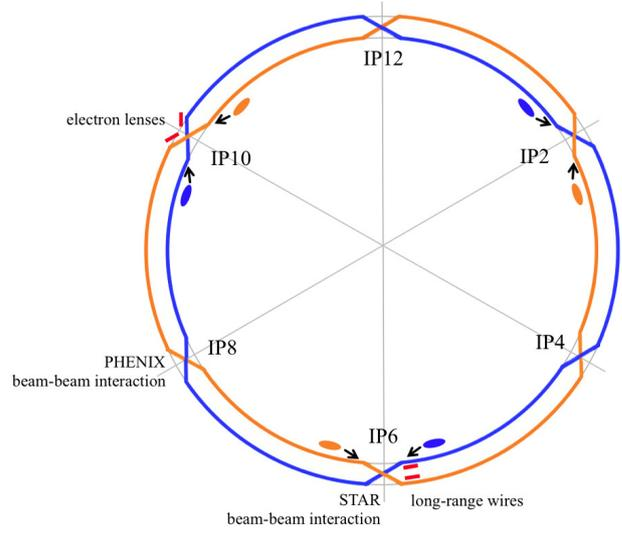
Figure 1: Beam-beam interactions in RHIC and locations of wires and electron lenses.
