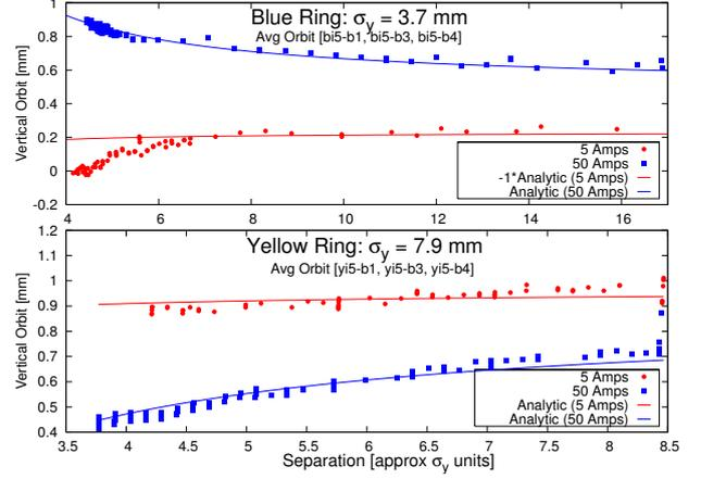
Figure 11: Vertical orbit change (average of 3 BPMs near wire) as a function of vertical distance, in Blue and Yellow ring at 5 A and 50 A. Solid lines in all plots represent the analytical prediction.
