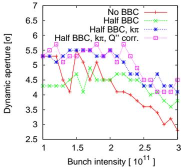
Figure 4: Dynamic apertures of half head-on beam-beam compensation with the betatron phase advance adjustment and the global second-order chromaticity correction.
