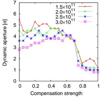
Figure 3: Dynamic apertures of four proton bunch intensities versus the head-on beam-beam compensation strength.
