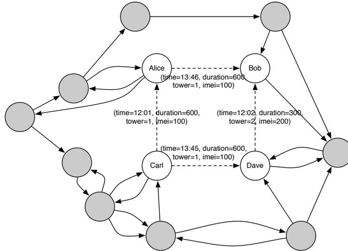
Figure 1: A partial example interaction graph for call data records, capturing the telephone calls among a set of people. To motivate our design, this paper will focus on a subgraph at a particular time range, indicated by the nodes colored white. Each edge in the graph is associated with attributes for the interaction, including the time the call was placed, the duration of the call, the cell phone tower, and the IMEI number identifying the device used.
