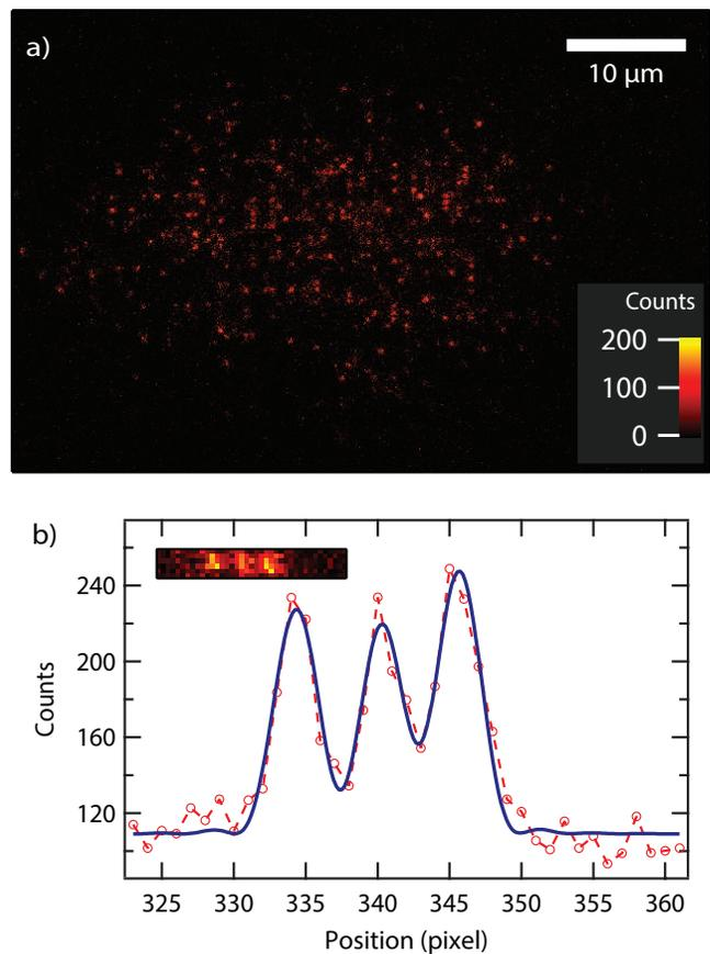
FIG. 4. (color online). a) False colored typical fluorescence image of atoms trapped in a two-dimensional optical lattice. One CCD camera count represents roughly  $1/8$  incident photons. b) Intensity profile along the center for three consecutive occupied lattice sites (inset image). Fitting using three point spreads function resulted in a resolution of  $377(13)$  nm. A single pixel represents  $90$  nm in real space.
