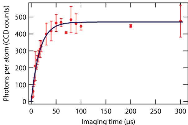
FIG. 5. Total photons per atom (in CCD counts) as a function of the cooling light exposure time. The profile is fitted using an integrated exponential decay, resulting in a life-time of 17(1)  $\mu\text{s}$ .
