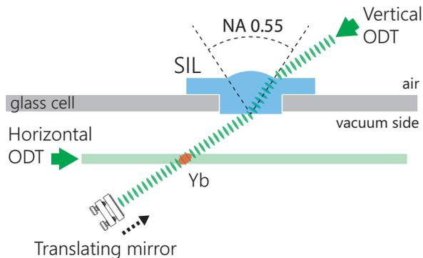
FIG. 2. (color online). Lateral view of the SIL attached to the 3 mm thick glass cell. Atoms are evaporated cooled in crossed-beam dipole trap. A “conveyor belt” generated by reflecting back the vertical ODT beam is used to transport the atoms closer to the surface.
