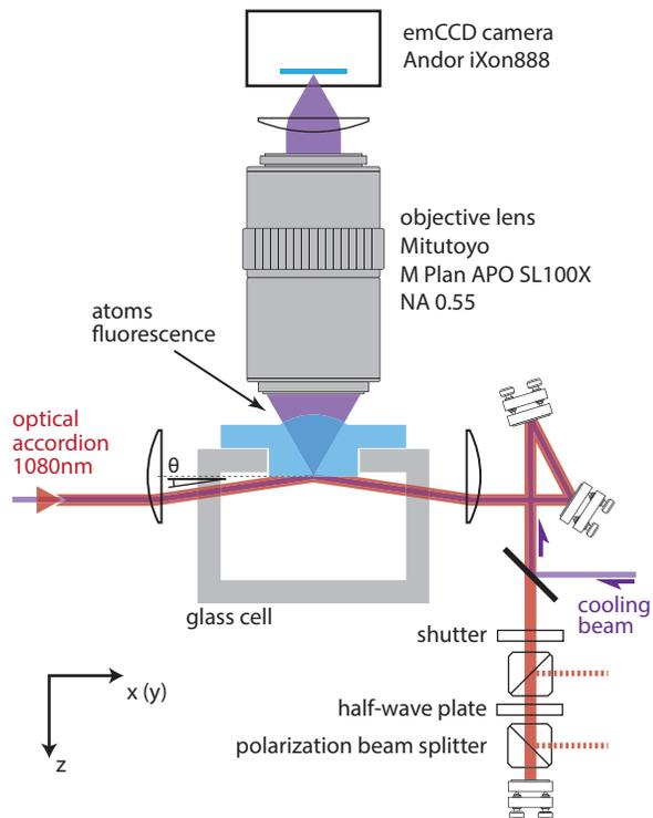
FIG. 3. (color online). Experimental apparatus to trap and image atoms in a two-dimensional optical lattice. The microscope system is formed by an objective lens with a NA of 0.55, that combined with a SIL improves the NA of the system to 0.81. A retro-reflected optical accordion is used to create the two dimensional optical lattice.
