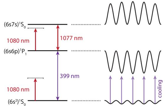
FIG. 1. (color online). Cooling mechanism for atoms trapped in an optical lattice. The lattice light at 1080 nm is near resonant with the upper  $^1P_1$ - $^1S_0$  transition (natural linewidth 3 MHz), creating a large light shift in the  $^1P_1$  state. The cooling beam is red detuned to the shifted  $^1S_0$ - $^1P_1$  strong dipolar transition (wavelength 399 nm, natural linewidth 29 MHz).
